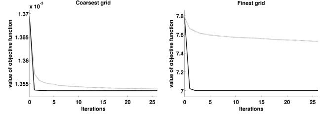
Figure 5. Representative performance of the minimization approach (32), (33) in a real scenario. The objective function is effectively minimized after few iterations at each resolution level (solid curve), as opposed to gradient descent that converges slowly (dashed curve).
