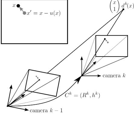
Figure 2. A scene point is defined by image coordinates  $x$  and depth  $d^k(x)$  in the coordinate system of camera  $k$ . Its projection moves by  $-u^k(x)$  to  $x'$  when the camera is rotated and translated backward by  $C^k = (R^k, h^k)$ .
