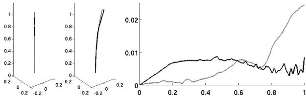
Figure 10. **Left&middle:** camera trajectories for *Avenue* and *Bend* sequences, resp., returned by VCT (gray) and our approach (black). The tracks are uniformly scaled to the overall camera movement (first to last frame). No rotational fitting was applied. **Right:** Euclidean distances between the trajectories, relative to the trajectory length. Differences are upper-bounded by 3%.
