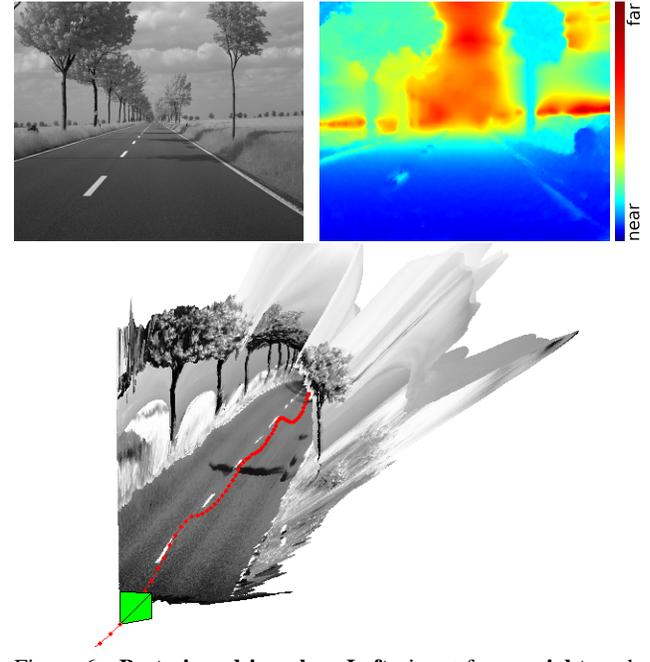
Figure 6. **Best viewed in color.** **Left:** input frame, **right:** calculated depth map, **bottom:** triangulation of the scene, camera position and direction (green camera symbol), camera track (red, dots indicate subsequent positions). Due to the moving trees, *homogeneous* sky regions *between* trees are naturally assigned to the trees (in terms of depth) in the temporal context, rather than to the horizon and in contrast to the center region.
