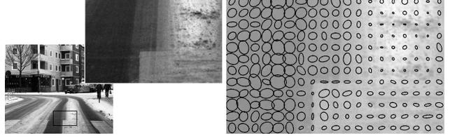
Figure 3. Detailed view of an image frame and an ellipse representation of the estimated flow uncertainty  $\Sigma_u^k(x)$ . Highly textured regions (upper right) can be correctly distinguished from locations with low confidence due to low signal-to-noise ratio (left) and image edges (aperture problem; middle).
