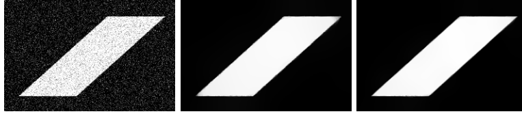
Fig. 1. 2D anisotropic TV filtering of artificial test image. Left: noisy test images, middle: filtering with the standard ROF model, right: anisotropic filtering with double directions. All images are scaled with respect to the intensity range of the original test image. Undesirable smoothing effects are considerably reduced on the right.
