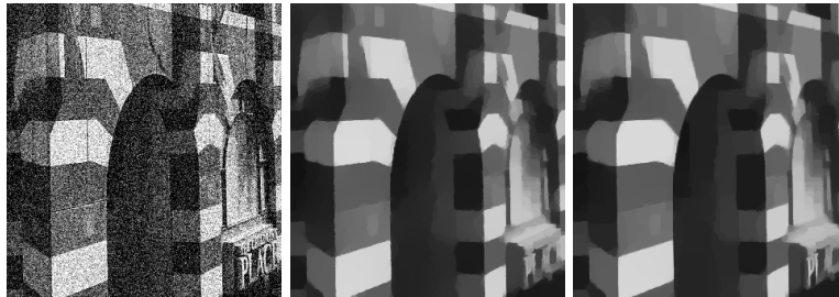
Fig. 2. 2D anisotropic filtering of real-world test image. Left: noisy test images, middle: result of standard ROF minimization, right: result of anisotropic TV minimization with double directions. Undesirable smoothing effects are considerably reduced on the right, see Fig. 3 for detailed views.
