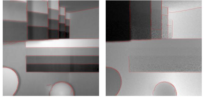
Fig. 5. Edge pixels without shadows in intensity data before (left) and depth data after (right) removing texture edges.
