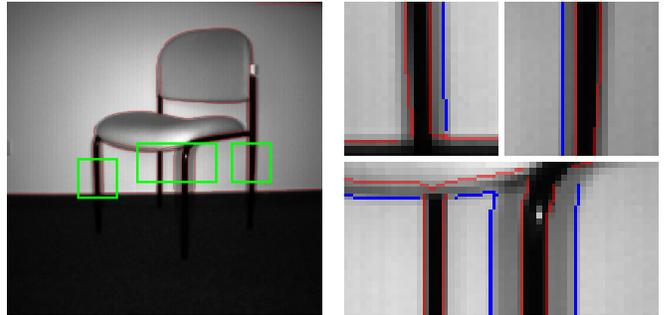
Fig. 3. Edge pixels in intensity data and closeups with highlighted shadow edges in blue.
