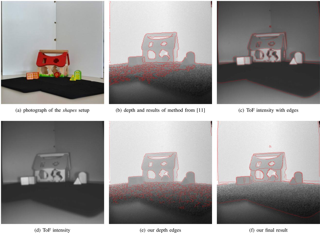
Fig. 9. Our method (f) performs better than (b) in noisy areas and at small depth steps, like the wooden bricks left and right of the house.
