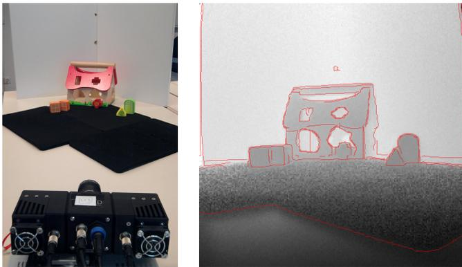
Fig. 1. Photograph of test setup (left) and result of our proposed method (right) as overlay to depth data. (All figures contain color. Please refer to the electronic version of the paper.)
