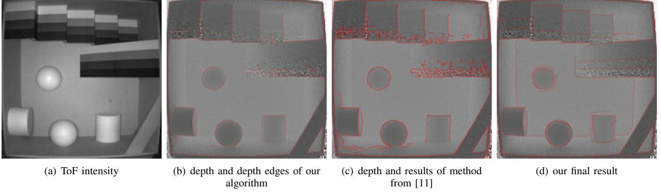
Fig. 8. The gain of our proposed approach in (c) compared to (b) can be seen clearly at the noisy regions as well as at the edges between the sides and the back of the *box*.
