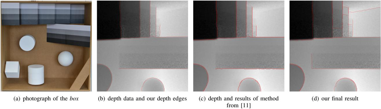
Fig. 7. If we compare (c) and (d), the main improvement are the detected ridge edges at the cost of a few texture edges.
