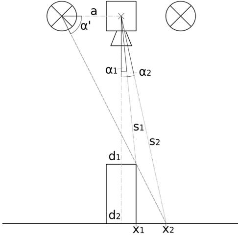
Fig. 4. Geometry of camera and light paths.
