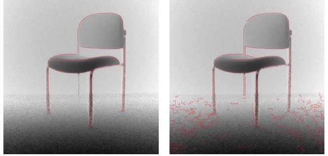
Fig. 2. Edge pixels in depth data with high (left) and low (right) thresholds.
