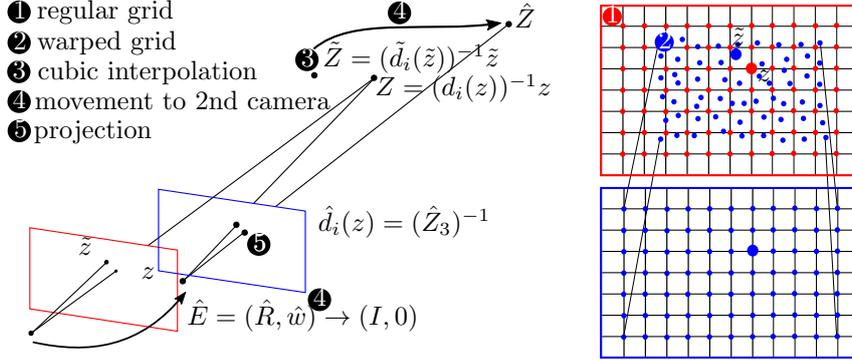
Figure 1: Discrete propagation of the disparity map
