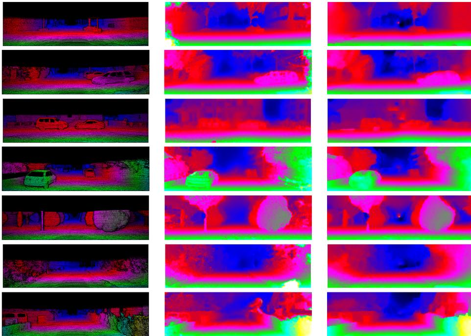
Figure 2: *Best viewed in color.* Reconstruction of the disparity maps; left column: ground truth from the KITTI stereo benchmark, middle column: monocular method of Becker et al. [1], right column: reconstruction with our monocular method. Although in the quantitative evaluation both methods perform equally, one can recognize that our method results in sharper corners. Due to spatial regularization [1] reconstructs regions close to the epipole better.
