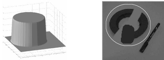
**Fig. 5. Left:** The labeling function  $L$ , shown in a 3D plot, indicates the area around the familiar object in which the prior should be applied ( $L = 1$ ) and the remainder of the image plane, which should be segmented according to the gray value information only ( $L = -1$ ). **Right:** Zero crossing of  $L$  superimposed on the input image.
