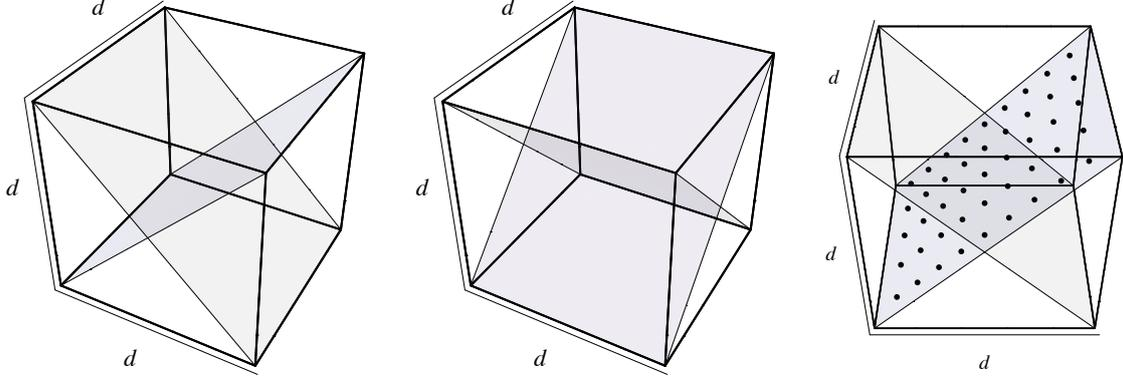
Figure 3. Imaging setup with four cameras corresponding to the image planes shown as two pairs in the left and center panel respectively. Right panel: Cell centers projected onto the first image plane are shown as dots for the case  $d = 5$ . The cube  $\Omega = [0, d]^3$  is discretized into  $d^3$  cells and projected along  $4 \cdot d(2d - 1)$  rays.
