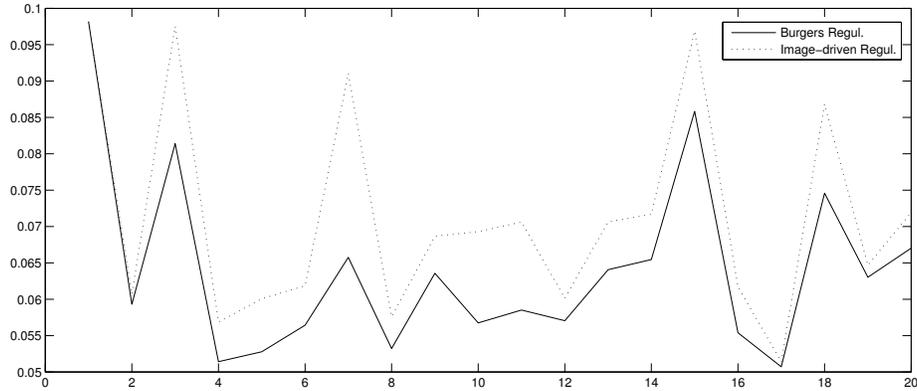
**Fig. 8.** Comparison of the  $L^2$  motion error between the purely spatial image-driven variational approach (3) and the approach (1) together with (5). The latter combination allows for temporal regularization with a recursive computational architecture, leading to consistently lower estimation errors if actual and expected motions agree (parameters:  $\alpha = 0.01$ ,  $\beta = 0.001$ ).
