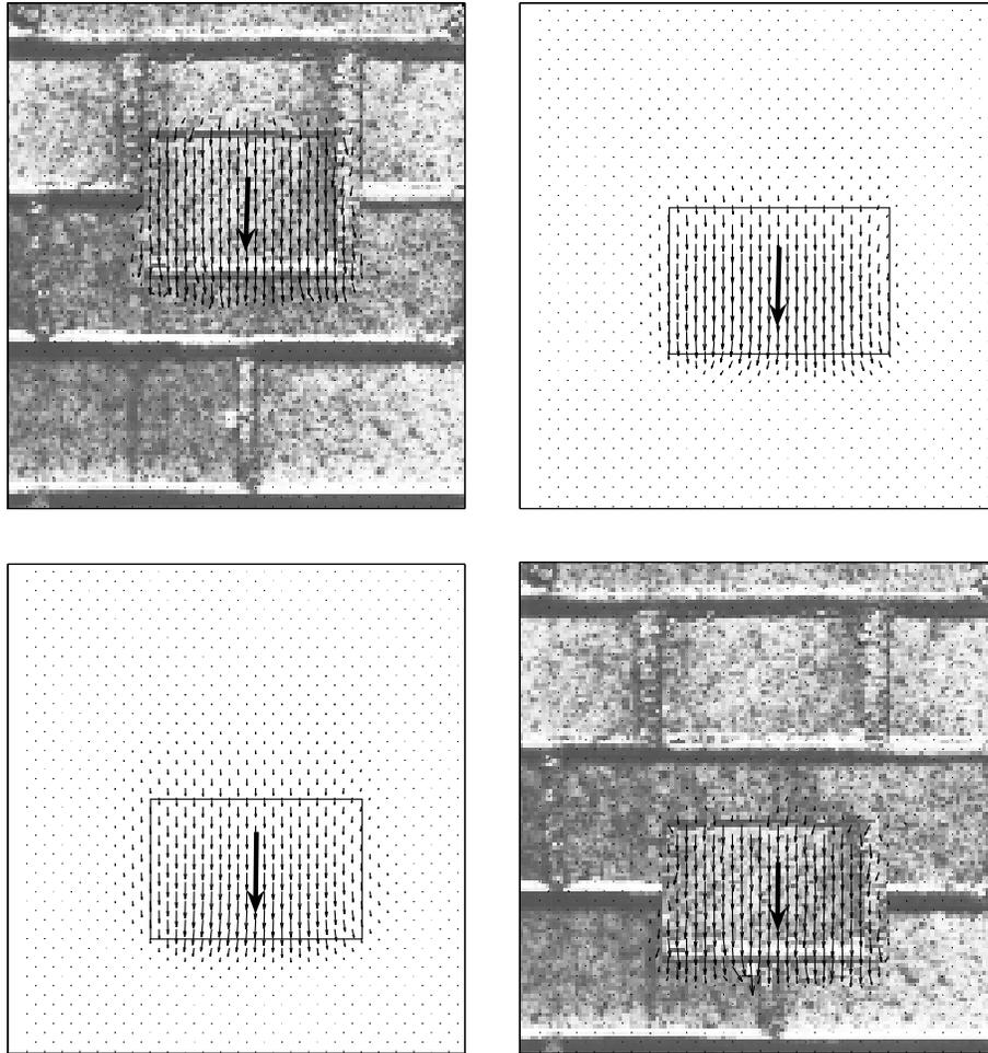
**Fig. 6.** Flow field estimates for an image sequence with three frames masked out. Because inertia of the fictive material allows for motion prediction, loss of data is immaterial (parameters:  $\alpha = 0.01$ ,  $\beta = 0.001$ ).
