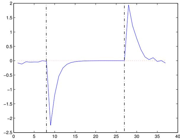
**Fig. 4.** A section through  $f$  ( $y$ -axis) over 37 frames ( $x$ -axis) corresponding to the image sequence shown in fig. 3. Vertical lines mark the frames where the object started and stopped, respectively. Signal peaks could be used to focus attention of a superordinate processing level. The fading characteristic is reminiscent of motion aftereffects (parameters:  $\alpha = 0.01$ ,  $\beta = 0.001$ ).
