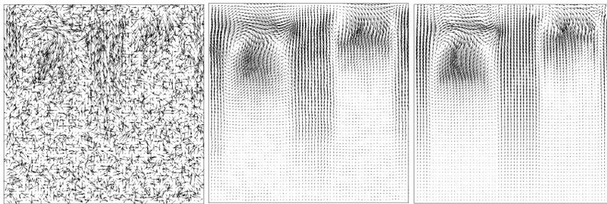
**Fig. 2** Vertical cross-sections of the velocity fields through the centers of convective cells. These vector fields correspond to the vorticities shown in Figure 1: noisy input (left), denoised result (center), ground truth (right).
