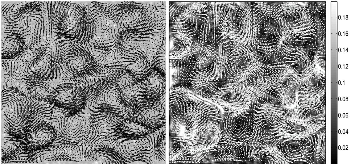
**Figure 3. Left:** 100th frame of the synthetic image sequence with ground truth velocity field. **Right:** Estimated velocity field for the 100th frame. The background intensity shows the absolute RMS error (brighter = larger error), which is about 0.055 px. on average (cf. fig. 4).
