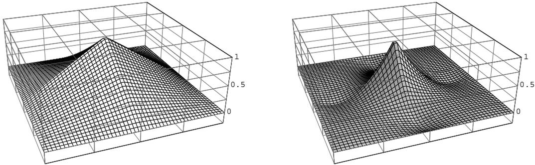
**Figure 2. Left:** Basis function  $\phi$  of a bilinear finite element. **Right:** Basis function  $\psi$  of a biquadratic finite element.
