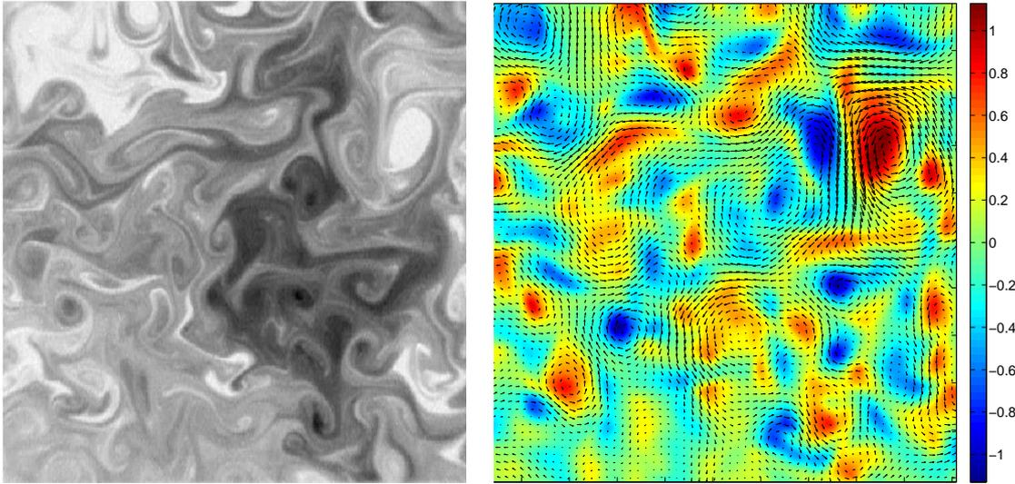
**Figure 7. Left:** Sample Real-World Passive Scalar Image (frame 80, size:  $512 \times 512$ .) **Right:** Recovered Velocity Field (with color-coded vorticity) with Vorticity Transport Approach.
