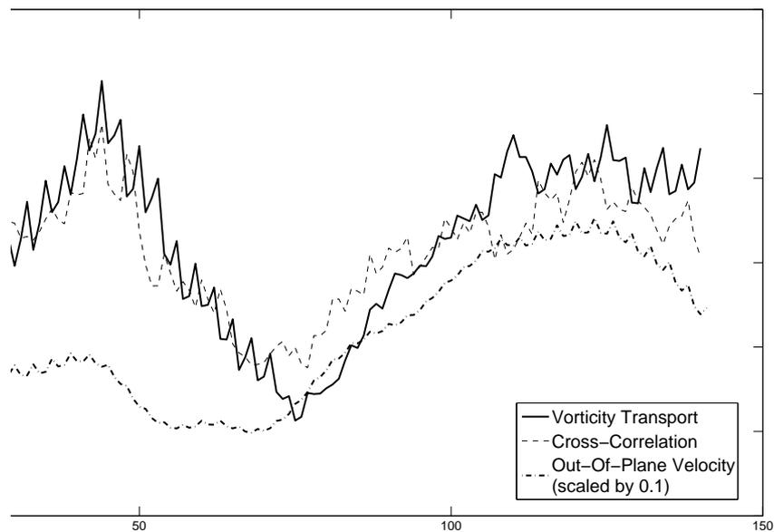
**Figure 6.** Average absolute RMS error (in pixels) for frames 1-140 of the VSJ 301 image sequence, using cross-correlation and novel optical flow technique with spatio-temporal regularization (with modification of sec. 3.3). Both approaches have similar accuracy.
