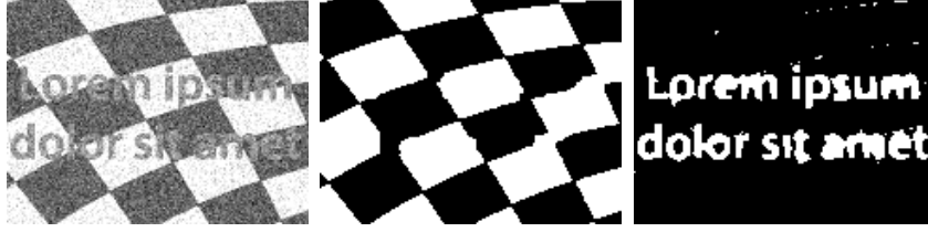
Figure 7. Simultaneous segmentation and background reconstruction by solving a single convex optimization problem within our framework. Left: Noisy image (PSNR = 20.82 dB). Center: Reconstructed background. Right: Extracted foreground. The image was segmented into four classes, and a (non-Euclidean) d was chosen so as to differentiate text over dark and light background.
