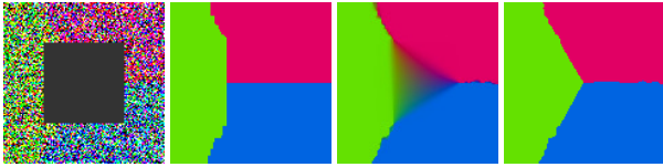
Figure 4. Region filling capabilities of the proposed method. Left: Input image (PSNR = 3.67 dB) with blanked-out (data term set to zero) square. Second from left: Result of the alpha-beta swap benchmark code from [20]. Second from right and right: Result of our algorithm with Potts distance before and after binarization. While the continuous energy does not promote a true binary solution in this case, after binarization the result conforms to the continuous framework. The alpha-beta swap minimizes an anisotropic energy, which leads to blocky artifacts.
