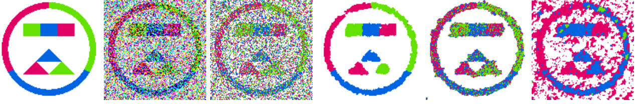
Figure 3. Four-class color segmentation using our method with varying distance. Left to right: Groundtruth; groundtruth with Gaussian noise ( \sigma = 1 ) and clamped to [0, 1] (PSNR = 5.81 dB); purely local labeling without regularizer; proposed method with Potts, fg-bg, and linear distance. The fg-bg distance was chosen to clearly segment the three foreground classes (colors) from the background class (white), but allow for a large variance between foreground classes. The linear distance, which implies an ordering of the labels, corresponds to a degenerate embedding and results in a strongly suboptimal discrete solution.
