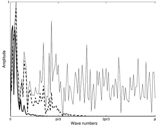
Fig. 1. Velocity spectra of an original turbulent fluid flow (thick solid line), the flow corrupted by noise (fine solid line), and the flow after solenoidal projection (8), (7) and Gaussian lowpass filtering (10) (dashed line). Although noise has been effectively removed, a significant nonphysical component of the fluid flow estimate remains—cf. Fig. 2, bottom, and Fig. 3, top.
