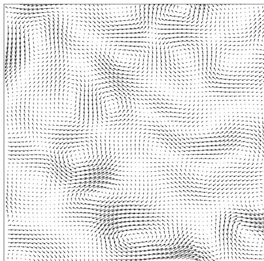
Fig. 8. Vector field resulting from TV-denoising. The corresponding error measurements are SDR = 1.96, ADR = 2.07, DDR = 0.65, NDR = 2.48.
