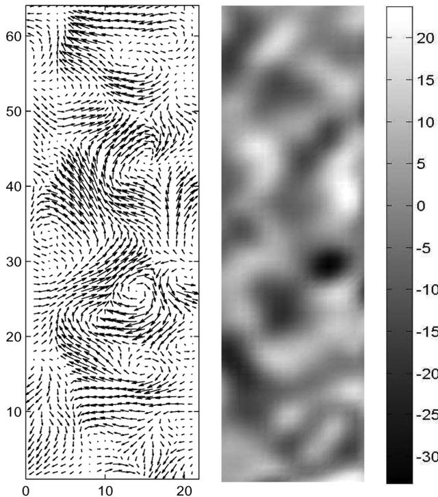
Fig. 11. VTE-based data restoration. Left: Velocity vector field. Right: Vorticity field.
