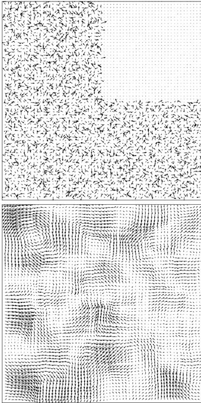
Fig. 2. Top panel: Noisy input field. The original data field without noise is shown in the upper right quadrant to illustrate the signal-to-noise ratio. Bottom panel: The data field after filtering using the Gaussian filter. Although noise has been effectively removed, a significant nonphysical component of the fluid flow estimate remains—cf. Fig. 3, top.
