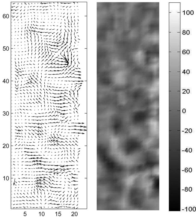
Fig. 10. Measured data. Left: Velocity vector field. Right: Vorticity field.
