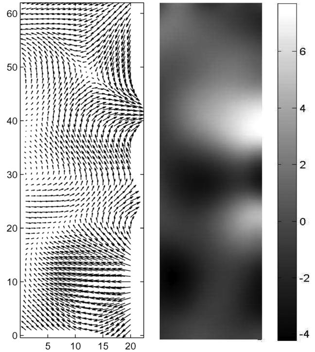
Fig. 12. TV-based data reconstruction. Left: Velocity vector field. Right: Vorticity field.
