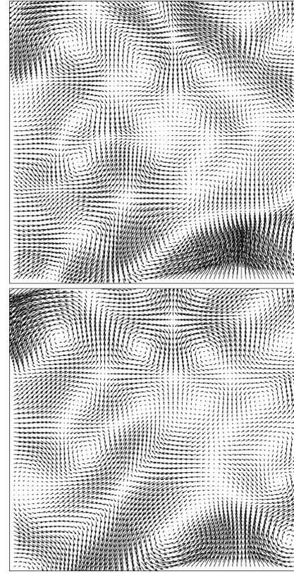
Fig. 3. Top panel: Restored flow corresponding to Fig. 2 but after the complete cycle of four computational steps of the overall approach. Bottom panel: Ground truth vector field.
