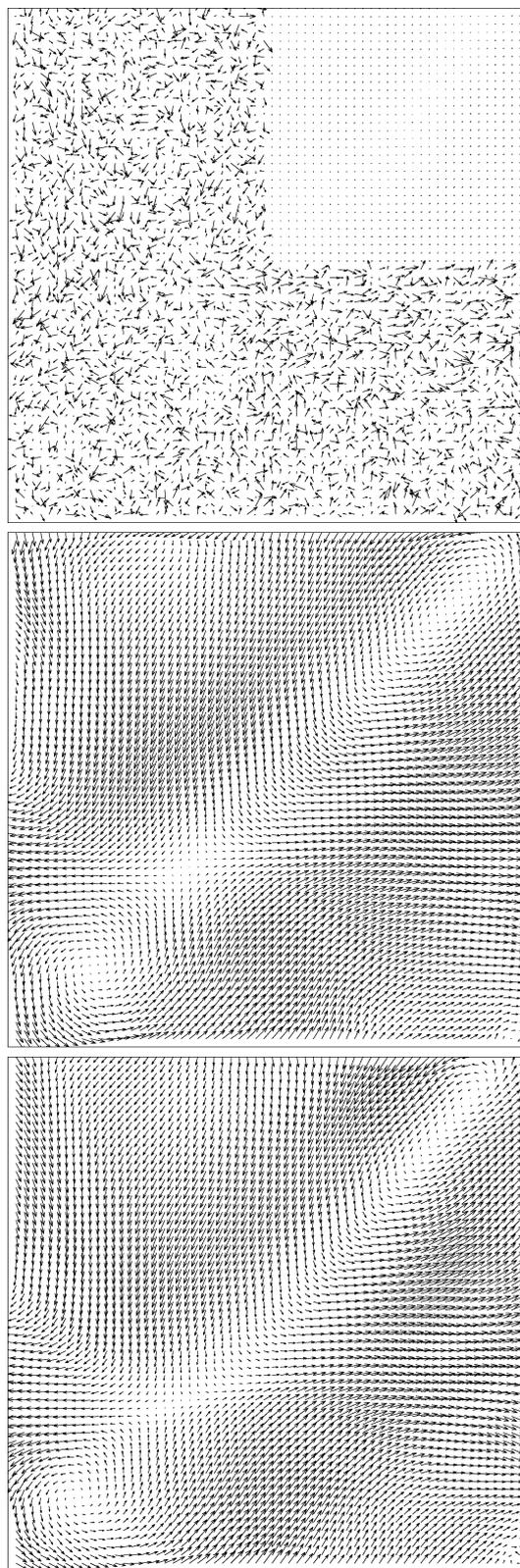
Fig. 4. Top: Noisy input  $\mathbf{d}$ . Noise has been cut out within a rectangular region to illustrate the signal-to-noise ratio. Middle: Denoised data  $\mathbf{u}$ . Bottom: Ground truth flow  $\mathbf{g}$ . Performance measures:  $SDR = 4.34$ ,  $ADR = 3.046$ ,  $NDR = 2.12$ ,  $DDR = 0.82$ .
