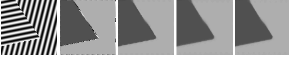
Figure 5: Left to right: (a) Synthetic image with oriented textures, inspired by [33]. (b) Local orientations computed via derivatives of Gaussians. Orientations have been mapped to grey-values. Note that the orientations represented by black and white are close neighbours. (c) Orientations after median filtering of the orientation matrices with Frobenius norm and a disk-shaped structure element of diameter 7. (d) Same with structure element of diameter 9. (e) Spectral norm median filtering, diameter 9. From [35].
