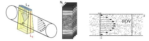
**Fig. 1.** A schematic representation of an Echo PIV setup. The left image, adapted from [2], overviews geometry and orientation of the transducer. Velocity is estimated from a sequence of B-mode images (middle). Flow motion is estimated from the motion of tracer particles injected in the medium (right), which follow the flow dynamics – here, a steady laminar flow.
