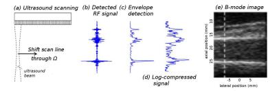
**Fig. 2.** B-mode imaging in Echo PIV: images are not recorded as snapshots, but are usually constructed line-by-line, due to the shifting of the ultrasound beam (a). The data – RF signals (b) – can be converted (offline) to so-called B-mode images (e) by means of envelope detection (c) and log compression (d). This scanning procedure results in a blurred, smeared image due to moving particles between consecutive measurements.
