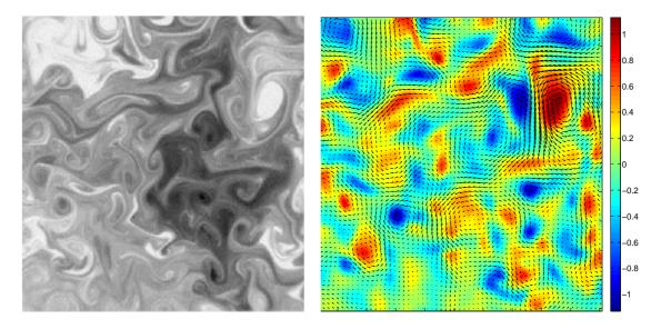
Figure 7. Left: Sample Real-World Passive Scalar Image (frame 80, size:  $512 \times 512$ .) Right: Recovered Velocity Field (with color-coded vorticity) with Vorticity Transport Approach.
