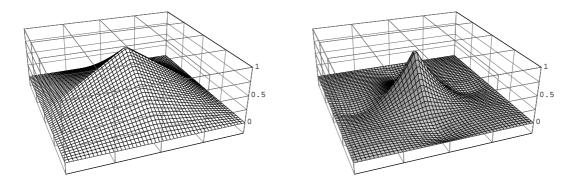
**Figure 2. Left:** Basis function  $\phi$  of a bilinear finite element. **Right:** Basis function  $\psi$  of a biquadratic finite element.
