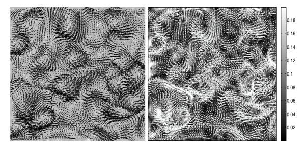
Figure 3. Left: 100th frame of the synthetic image sequence with ground truth velocity field. **Right:** Estimated velocity field for the 100th frame. The background intensity shows the absolute RMS error (brighter = larger error), which is about 0.055 px. on average (cf. fig. 4).
