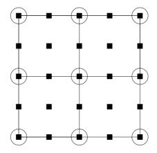
**Figure 1.** Sketch of 2D Taylor-Hood elements: biquadratic velocity elements (squares) and bilinear pressure elements (circles).
