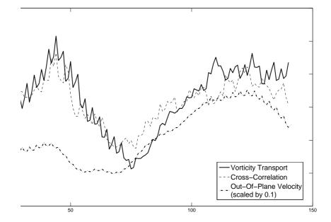
Figure 6. Average absolute RMS error (in pixels) for frames 1-140 of the VSJ 301 image sequence, using cross-correlation and novel optical flow technique with spatio-temporal regularization (with modification of sec. 3.3). Both approaches have similar accuracy.
