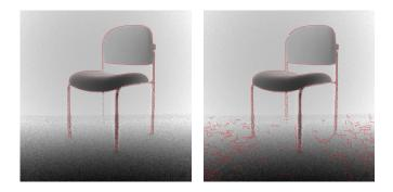
Fig. 2. Edge pixels in depth data with high (left) and low (right) thresholds.
