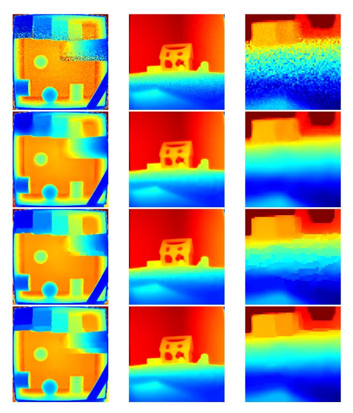
Fig. 10. Denoising depth data. Original depth image (top row), denoising as described in [12] (second row), anisotropic TV with edges calculated with algorithm described by Lejeune et al. [11] (third row) and with edges from the proposed approach (bottom row). The third column is a close-up of the second column with enhanced contrast. We observe better quality of the denoised depth map (sharpness of edges, regularity of faces) using the edge information of the proposed algorithm.
