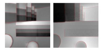
Fig. 5. Edge pixels without shadows in intensity data before (left) and depth data after (right) removing texture edges.
