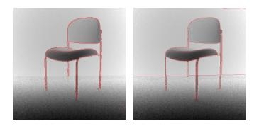
Fig. 6. Edge pixels on depth data, calculated with method from  $\left[11\right]$  (left) and our final result (right)
