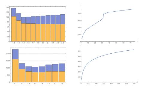
FIGURE 5.9. The inexact accelerated FBS algorithm for the *nonnegativity constrained* problem (1.4). LEFT: Relation of the number of outer iterations (not scaled down) and the *total* number of inner iterations (scaled down by 1/1000) as a function of the exponent q of the error  $\varepsilon_k = \mathcal{O}(k^{-q})$  (4.17). RIGHT: The number l of inner iterations at each outer iteration k, for exponents q = 1.8 (top) and q = 2.0 (bottom) of (4.17).
