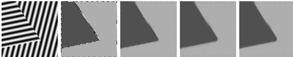
Figure 5: Left to right: (a) Synthetic image with oriented textures, inspired by [33]. (b) Local orientations computed via derivatives of Gaussians. Orientations have been mapped to grey-values. Note that the orientations represented by black and white are close neighbours. (c) Orientations after median filtering of the orientation matrices with Frobenius norm and a disk-shaped structure element of diameter 7. (d) Same with structure element of diameter 9. (e) Spectral norm median filtering, diameter 9. From [35].
